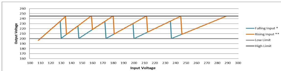
\*Falling input: Output Voltage graph, when the input voltage goes down
