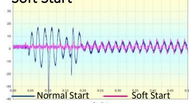
Reduces the load and Torque and electric current surge during startup. This reduces the mechanical stress on the motors and their components as well as electrical stresses on winding and cables, thus extending the lifespan of the system.
